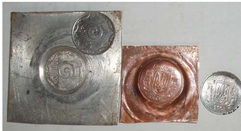
Fig. 13 General view of a coin stamped on aluminum and copper samples. Notice reproduction of fine details of the coin on the sample surface
